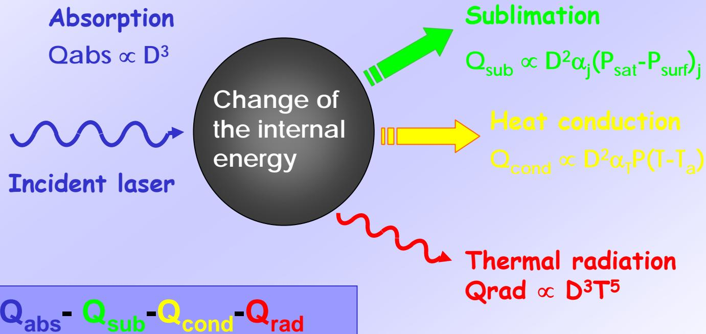
The LII signal is based on the energy and mass balance between a single particle and its surrounding
