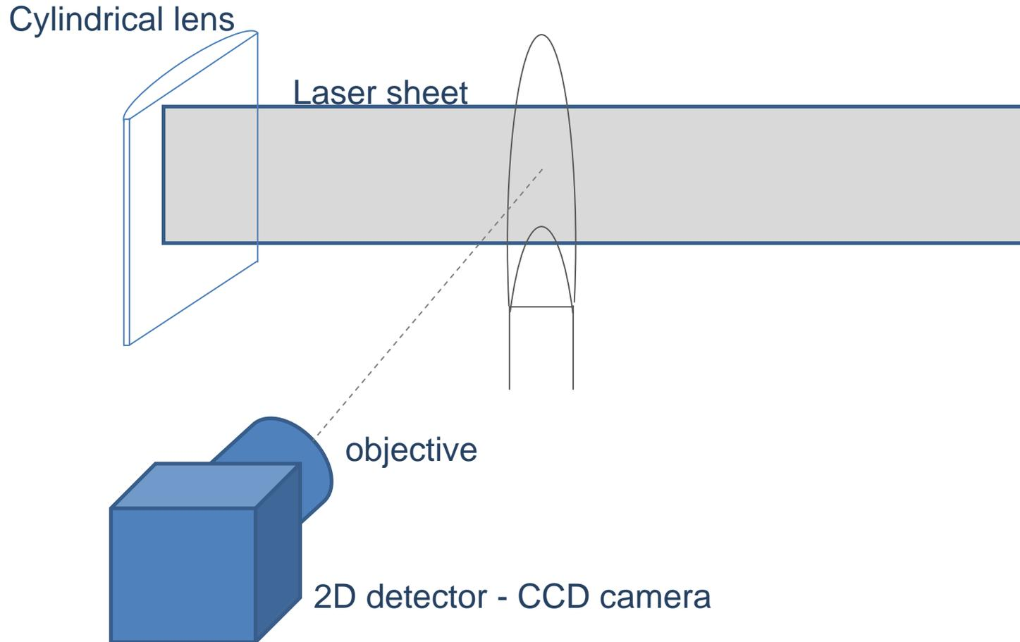
Laser beam: from circular section to a vertical sheet using a cylindrical lens
