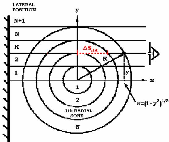
Tomographic deconvolution by 3-point Abel inversion and iterative method for self-absorption correction
