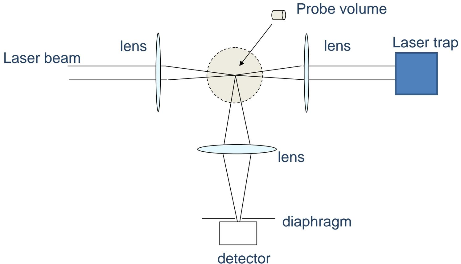
Probe volume: interception of the laser beam and the image of the detector slit in the flame. Diameter depends on the laser wavelength, the focal lens and the beam diameter.
