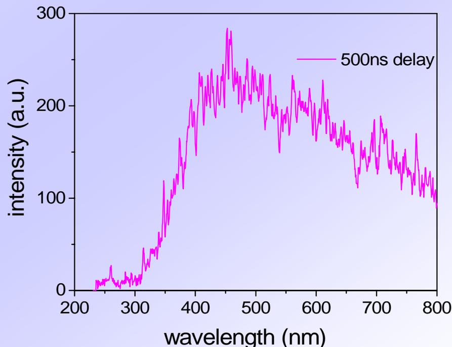
just after the laser pulse the maximum signal is at short wavelengths (higher temperature) but...
