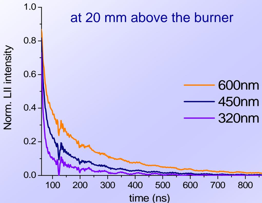
...at longer wavelengths the signal drops more slowly allowing better SNR at longer times
